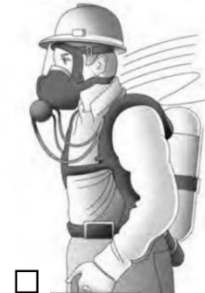
Full Facepiece Self-Contained Breathing Apparatus (SCBA) Pressure demand mode is APF=10,000 Needs to be fit tested
