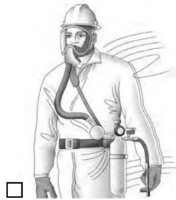
Full Facepiece Supplied-Air Respirator (SAR) with an auxiliary Escape Bottle APF=1,000 APF = 10,000 (if used in "escape" mode) Needs to be fit tested
