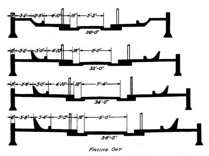
Fig. 6.—Typical sections showing plan for cows facing in or cows facing out in barns of different widths. A 34-foot width is a very common one, though a 32-foot width is often used with satisfaction. (Refer to figure 16 for correct stall length for different breeds.)
