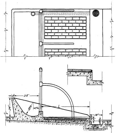
Fig. 17.—Stall plan and section, showing use of cork brick or creosoted wood-block flooring.
