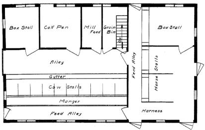
Fig. 4.—Typical floor plan of a small general-purpose barn.
