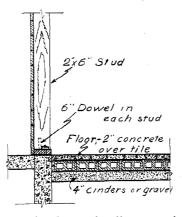
Fig. 28.—A grain bin, showing floor and wall construction. Bin floors should be dry and rat-proof. The walls should be well anchored to resist the thrust of several feet of grain.
