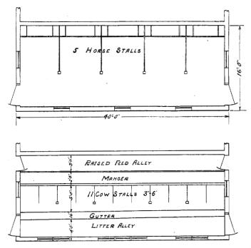
Frg. 38.—Remodeling suggestion. An unused stable may be converted into a well-arranged dairy section. Posts may have to be moved latterly to conform to new stall widths, but this shift usually can be made if an additional piece is added over the posts. Extra windows must be added, which can be done without disturbing those already in place.
