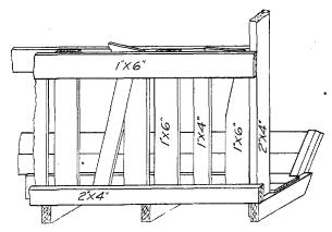
Fig. 25.—Calf stanchions and mangers of wood construction.
