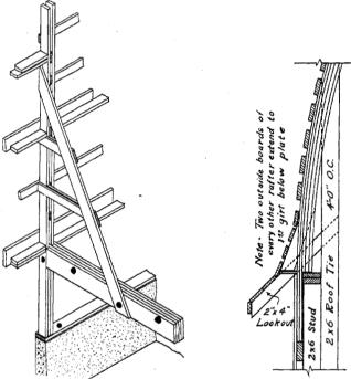
Fig. 14.—Girder and end wall construction.
