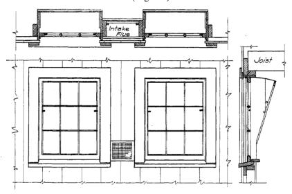
Fig. 22.—Nine-light windows, placed in pairs with intake ventilating flue between, is a very popular installation. Note the ventilating shield which deflects the air toward the ceiling when the window is tilted inward at the top, preventing direct draft on the cows. The window may be raised a few inches when in the open position so as to allow a direct draft for summer.
