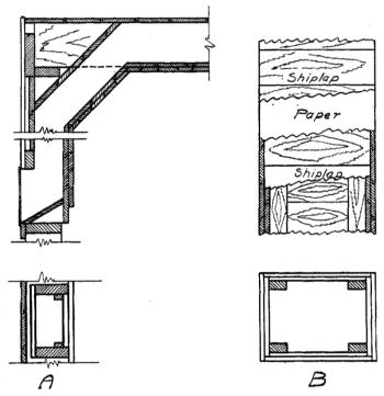
Fig. 24.—Details of ventilating flue construction. (A) Intake flue. (B) Out-take flue.
