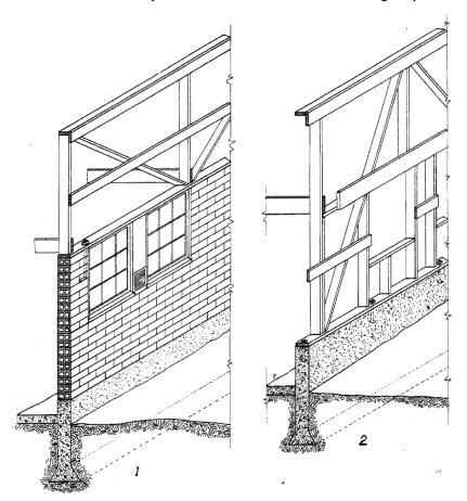
Fig. 8.—Concrete foundation with (1) tile wall and (2) frame wall.
