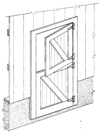
Fig. 21.—A Dutch door. This is a very convenient type of hinge door for feed alley or stock door. The top part may be left open for ventilation and if desired bars may be added to lower door to keep stock from reaching over it when the upper one is open.
