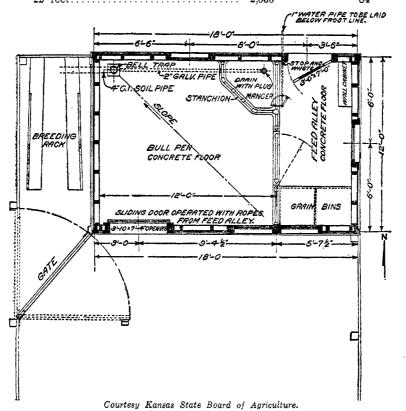
Fig. 37.—A bull pen outside the main dairy barn is usually most satisfactory. The plan shown is a suggested arrangement for bull shed, breeding rack, and lot.
