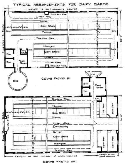
Fig. 5.—Typical floor plan arrangements for dairy barns—upper plan for cows facing in; lower plan for cows facing out.
