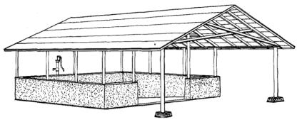
Fig. 32.—Covered concrete manure pit and shelter for spreader.
