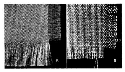
FIG. 14. — (A) Satin with silk warp and rayon filling, 55 percent cuprammonium, 45 percent silk. (B) Medium weight dress fabric of rayon and cotton ply yarns, 75 percent viscose, 25 percent cotton. (Magnification  $2 \times .$ )
