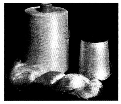
FIG. 4.—Rayon yarn shown in the shipping cone, spool and skein.
