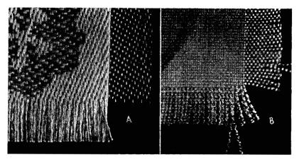
Fig. 11.—Tablecloths of viscose rayon and cotton. (A) Cotton warp and rayon filling. (B) Warp and filling of two-ply yarns, one of rayon and the other of cotton. (Magnification  $2 \times .$ )
