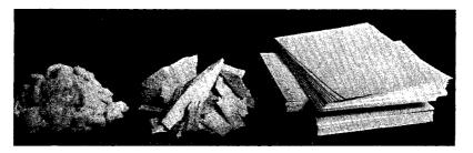
FIG. 1.—Cotton linters, spruce wood chips and wood pulp are the raw materials used in the production of rayon.
