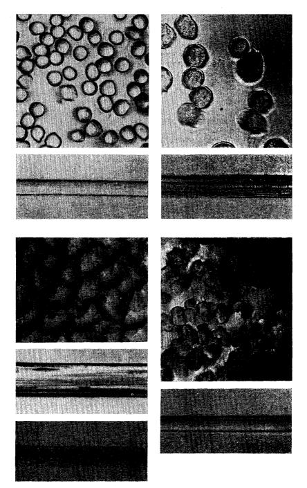
FIG. 8.—Photomicrographs of cross-section and longitudinal views of different synthetic fibers. Upper left—Cuprammonium. Upper right—Lanital. Lower left—Viscose, with longitudinal views of lustrous and delustered fibers. Lower right—Acetate. (All cross sections magnified 380 diameters. Longitudinal views 350 diameters.)
