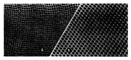
FIG. 7.-(A) Glass cloth used for draperies and (B) vinyon net used in shoes.
