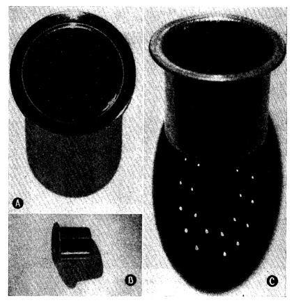
FIG. 3.—Spinnerettes used in "spraying" the synthetic solution. A and C are enlarged views, B shows an actual-sized view.
