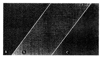
FIG. 10.—Specimens of spun rayon fabrics. A is acetate (Teca) herringbone twill; B is viscose rayon simulating linen; and C is a viscose gabardine.
