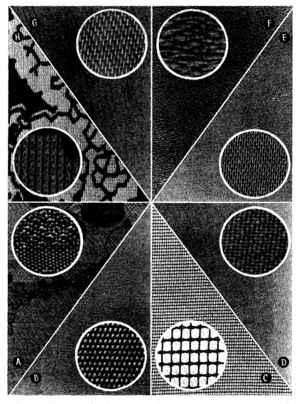
FIG. 5.—Fabrics made of continuous filament rayon: A, viscose crepe; B, viscose taffeta; C, viscose marquisette; D, cuprammonium twill; E, cuprammonium sheer; F, acetate granite cloth; G, acetate satin; H, acetate jersey. (Inserts magnified  $4 \times .$ )
