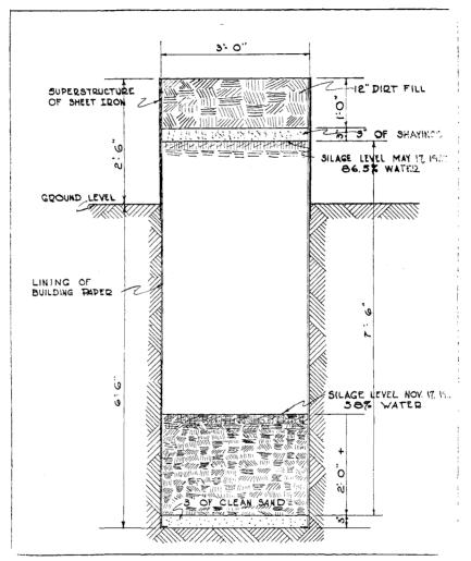
FIGURE 3.—Drawing shows size of pit silo and amount of settling of silage in six months. The grass settled from a depth of 7'6'' to 2'.
