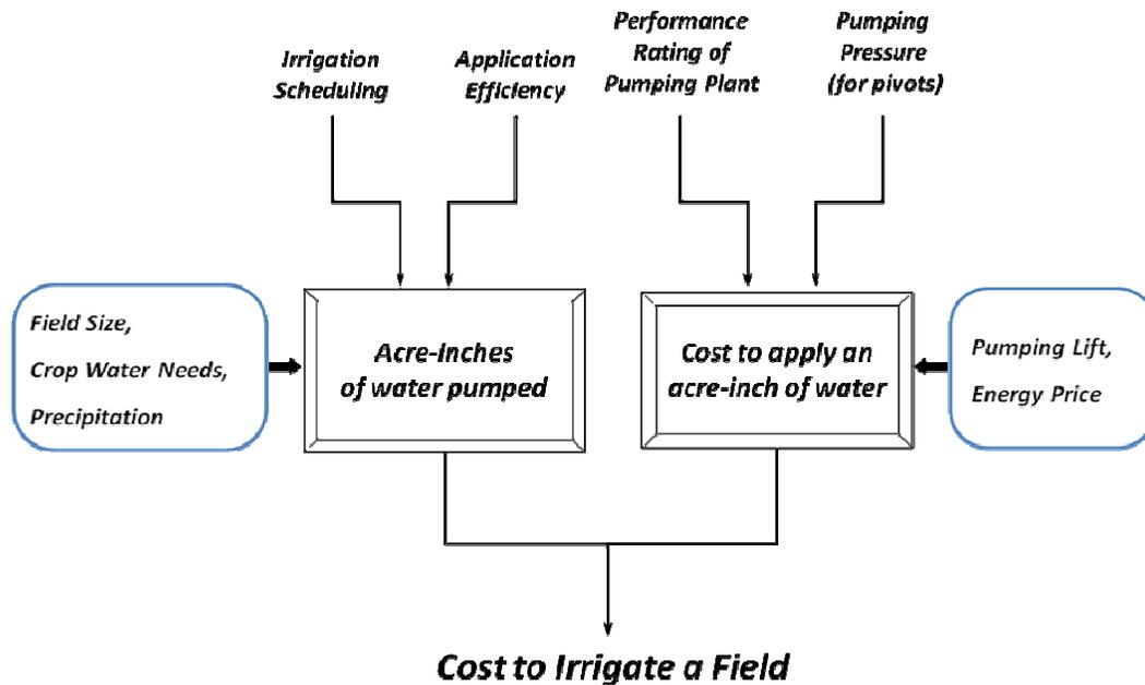
**Figure 1.** Diagram of factors affecting irrigation pumping costs.
