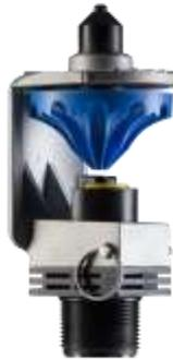
The R75 is a versatile, high-uniformity sprinkler. It features an easy to access nozzle, dual barrel spray plate for distance and uniformity, and adjustable stops to achieve the best arc of coverage. Its operating range is 25 to 60 PSI and can achieve a wetted radius of 70 feet. Six different nozzles will vary the flow from 24 to 69 GPM.
