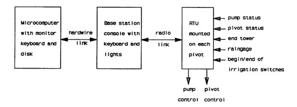
Figure 1 Schematic of radio control system
