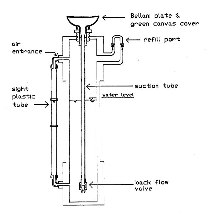
FIGURE 1. Schematic description of the modified atmometer.
