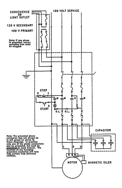
FIGURE 5. Schematic showing proper connection of power factor correction capacitors and control circuits.
