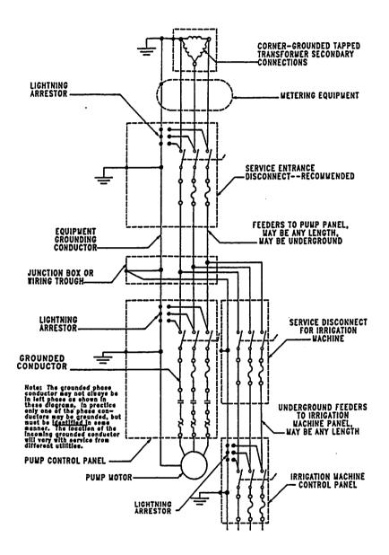
FIGURE 2. Schematic of a corner-grounded supply system for an irrigation installation showing the grounding and fusing for this type of supply.
