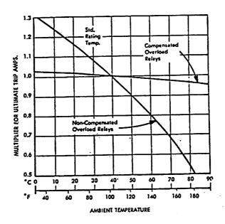
FIGURE 3. Ambient temperature effect on trip amps of ambient and non-ambient compensated overload relays.
