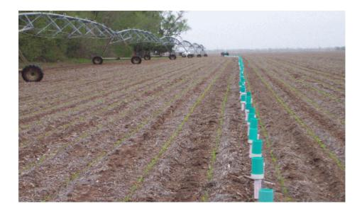
Figure 1. Series of IrriGages being positioned prior to an above canopy nozzle package evaluation.
