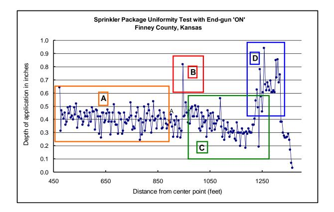
Figure 2. Uniformity test results for a Mobile Irrigation Lab uniformity evaluation (Rogers et al., 2008)
