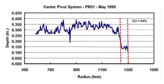
Figure 3. Unformity test results for a Mobile Irrigation Lav uniformity evaluation. (Rogers , unpublished data)
