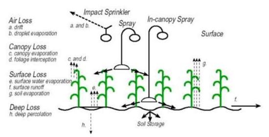
Figure 1: Illustration of where irrigation water losses can occur from KSU Extension Bulletin MF-2243, "Efficiencies and Water Losses of Irrigation Systems"
