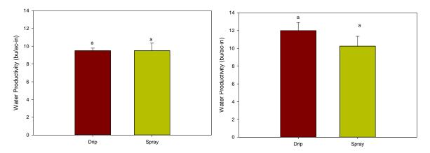
Figure 2. Water productivity of Mobile Drip Irrigation (Drip) and Low Elevation Spray Application (Spray) for irrigation capacity of 4.6 gpm/ac during the 2015 growing season at the Kansas State University SWREC, near Garden City, Kansas.
