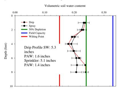
Figure 4. End of season soil water under Mobile Drip Irrigation (Drip) and Low Elevation Spray Application (Spray) for irrigation capacity 2.3 gpm/ac during the 2015 growing season at the Kansas State University Southwest Research-Extension Center, near Garden City, Kansas (Kisekka et al. 2017).
