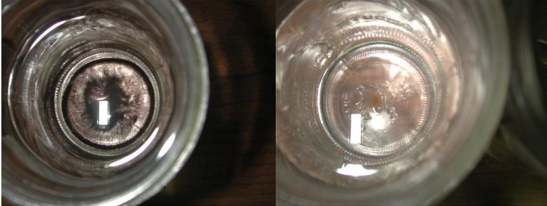
Figure 2. Jars containing Mn at 0.15 g material/gal of irrigation water, both at 0.125% H<sub>2</sub>O<sub>2</sub> concentration. The pH of the container on the left was 7.6; the pH of the container on the right was 6.5.
