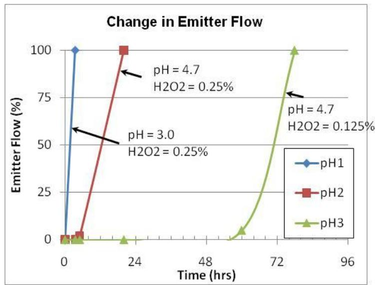
Figure 7. Relative emitter flow over time of clogged emitters treated with 0.25% H<sub>2</sub>O<sub>2</sub> at pH 3, 0.25% H<sub>2</sub>O<sub>2</sub> at pH 4.7, and 0.5% H<sub>2</sub>O<sub>2</sub> at pH 4.7 solutions with pressure at 30 psi.
