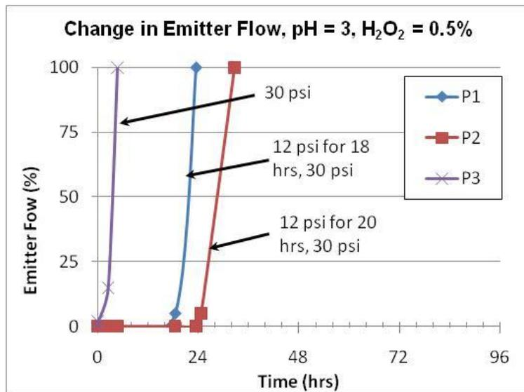
Figure 6. Relative emitter flow over time of three clogged emitters treated with a 0.5% H<sub>2</sub>O<sub>2</sub> solution at pH 3 and pressurized to 12 then 30 psi versus continuous 30 psi.
