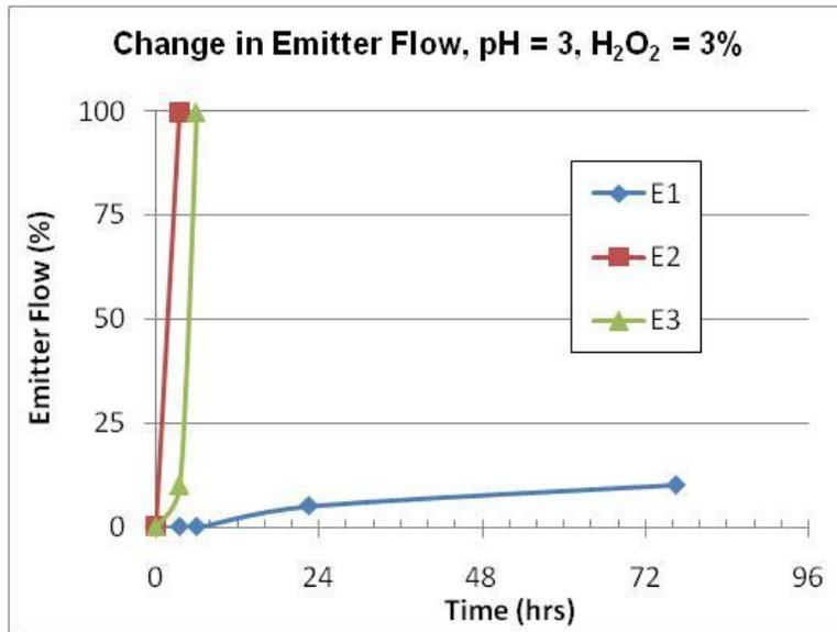
Figure 5. Relative emitter flow over time of three random clogged emitters treated with 3% H<sub>2</sub>O<sub>2</sub> solution at pH 3 and pressurized at 30 psi.
