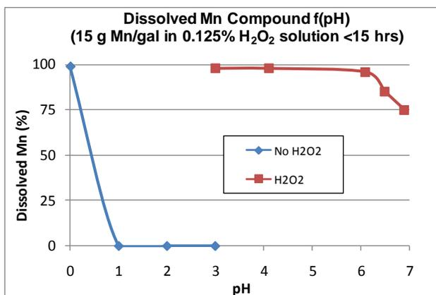
Figure 4. Percent of Mn material dissolved in solutions having pH ranging from 0 to 7, both with and without H<sub>2</sub>O<sub>2</sub> in the solution.
