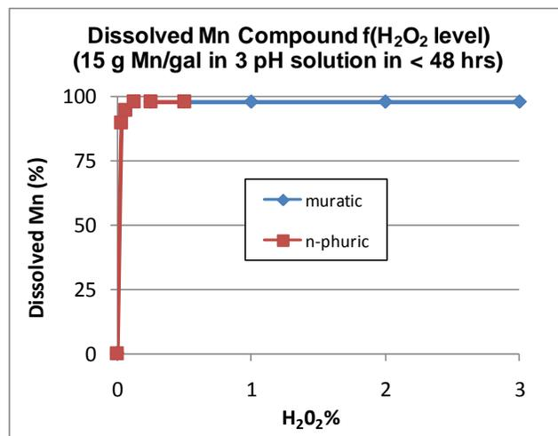
Figure 3. Percent of Mn material dissolved in solutions having H<sub>2</sub>O<sub>2</sub> concentrations of 0 to 3% using muriatic acid or N-pHuric to lower solution pH.
