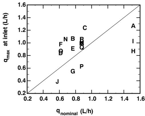
Figure 3. Maximum emitter discharge at the dripline inlet as related to the nominal emitter discharge specified by the manufacturer for 18 SDI systems evaluated in West Texas in 2008 and 2009. The letter symbols correspond to the 18 sites listed in table 1.
