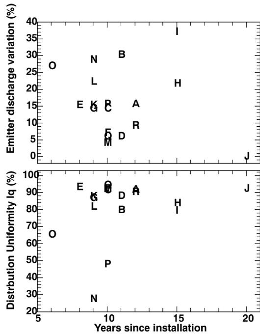
Figure 1. Emitter discharge variation and lower quartile distribution uniformity as affected by years since installation for 18 SDI systems evaluated in West Texas in 2008 and 2009. The letter symbols correspond to the 18 sites listed in table 1.
