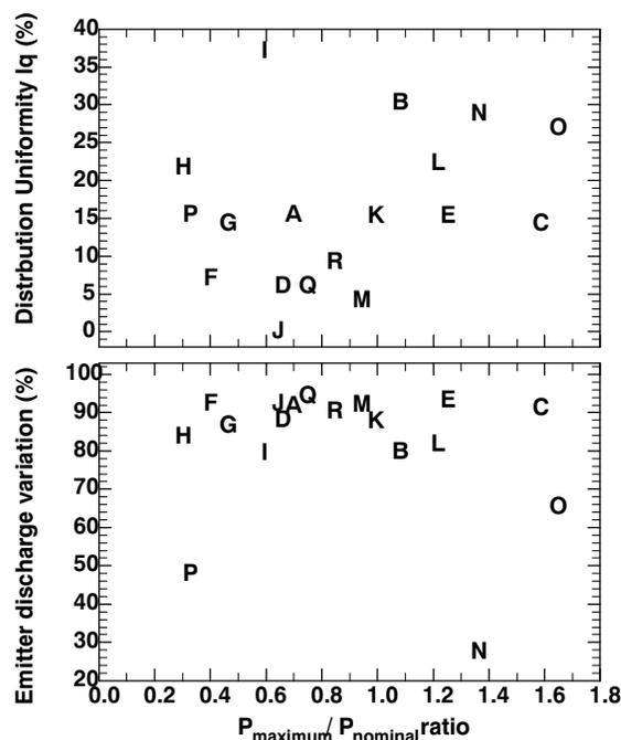
Figure 2. Emitter discharge variation and lower quartile distribution uniformity as affected by the ratio of the dripline inlet (maximum) pressure to the nominal design pressure specified by the manufacturer for 18 SDI systems evaluated in West Texas in 2008 and 2009. The letter symbols correspond to the 18 sites listed in table 1
