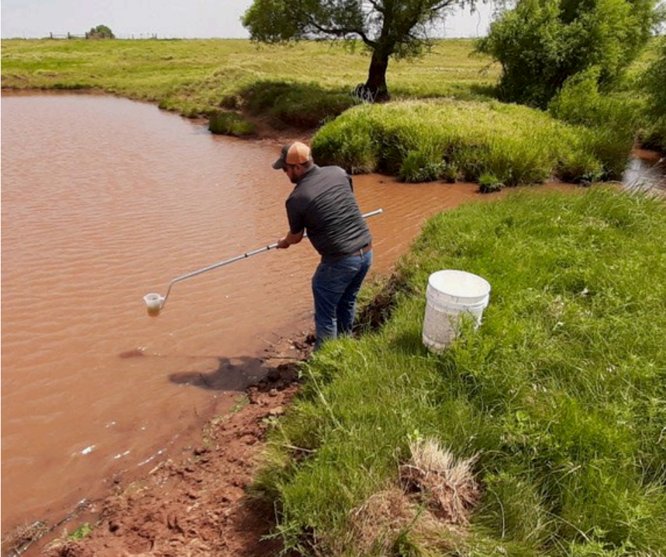
Figure 1: Dr. Joe Gerken sampling a pond in Harper County for blue-green algae.
