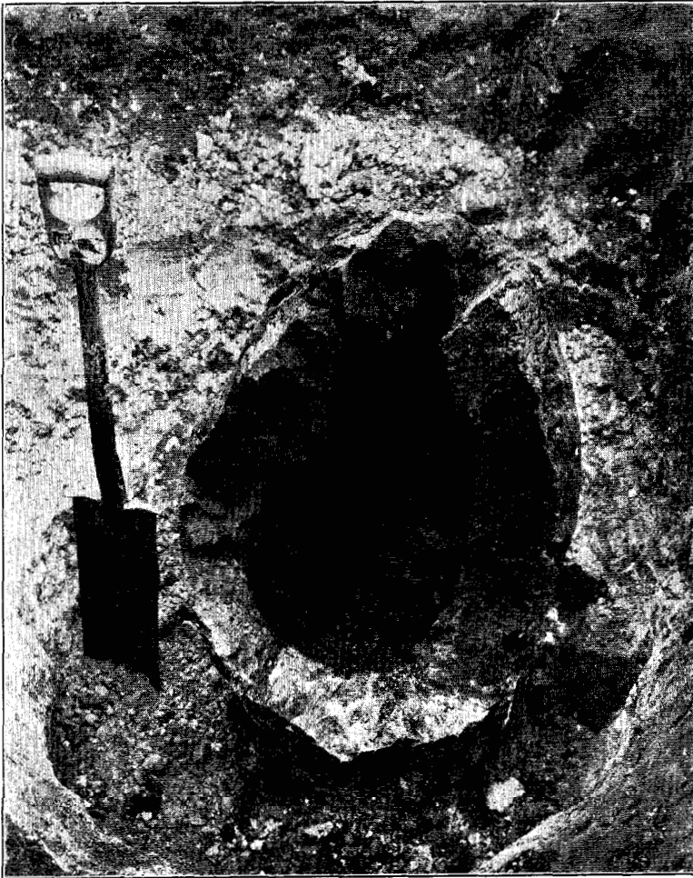
PLATE V.—A partly broken dynamite jug in Oswego Silt Loam soil, produced by one stick of 20 percent "Red Cross" powder placed in the soil at a depth of three feet. Photographed November 28, 1913. Cavity eighteen inches wide and twenty inches deep; thickness of walls varied from four to eight inches.
