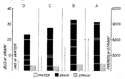
FIG. 10.—Graphs showing the effect of different quantities of irrigation water on yield of oats; average for five seasons, 1915 to 1919
