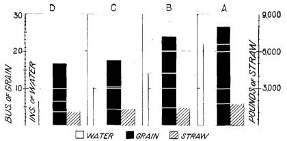
FIG. 11.—Graphs showing the effect of different quantities of irrigation water on yield of barley; average for five seasons, 1915 to 1919
