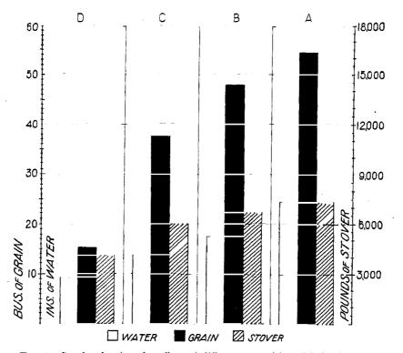
FIG. 4.—Graphs showing the effect of different quantities of irrigation water on yield of milo; average for four seasons, 1915 to 1918
