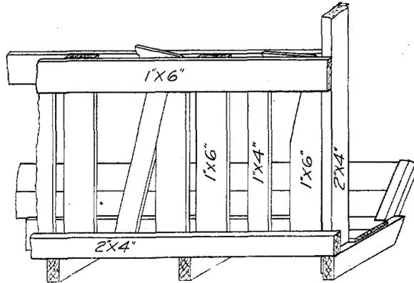
FIG. 25.—Calf stanchions and mangers of wood construction.
