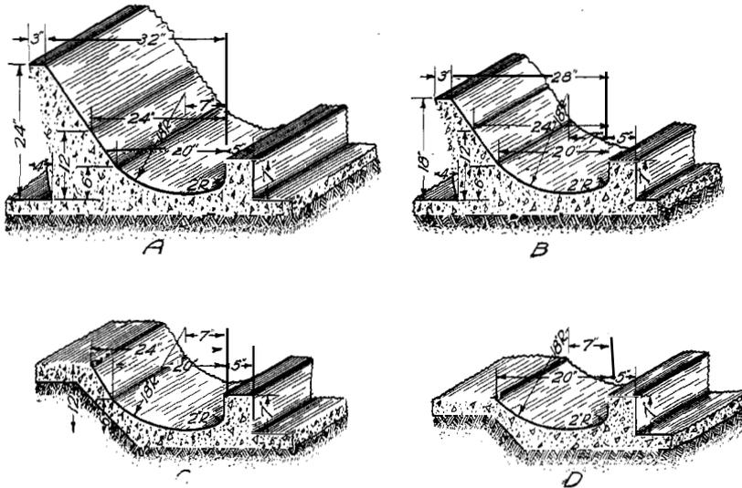
FIG. 18.—Standard manger sections. Mangers C and D are used only with raised feed alleys. Manger D is recommended only with lift mangers. These sections are the standard to which most manufacturers build their equipment.
