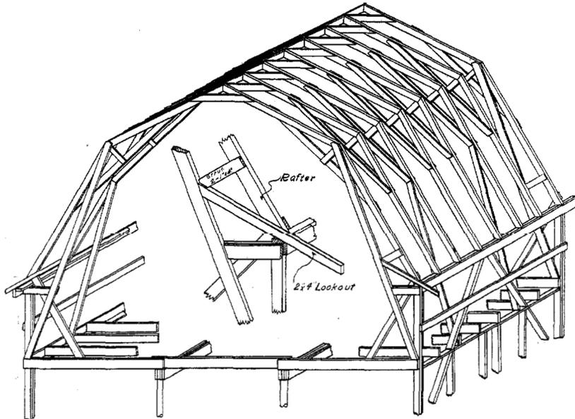
FIG. 12.—Braced rafter framing with detail of plate and foot of rafter.
