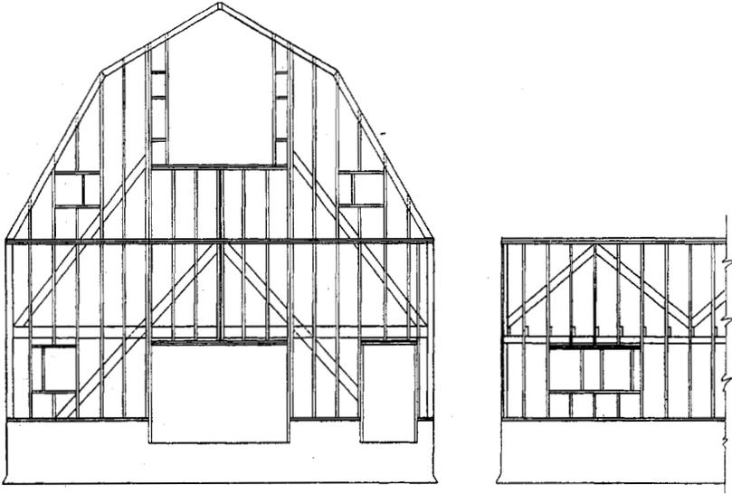
FIG. 9.—End and side wall framing and sway bracing for horizontal siding.
