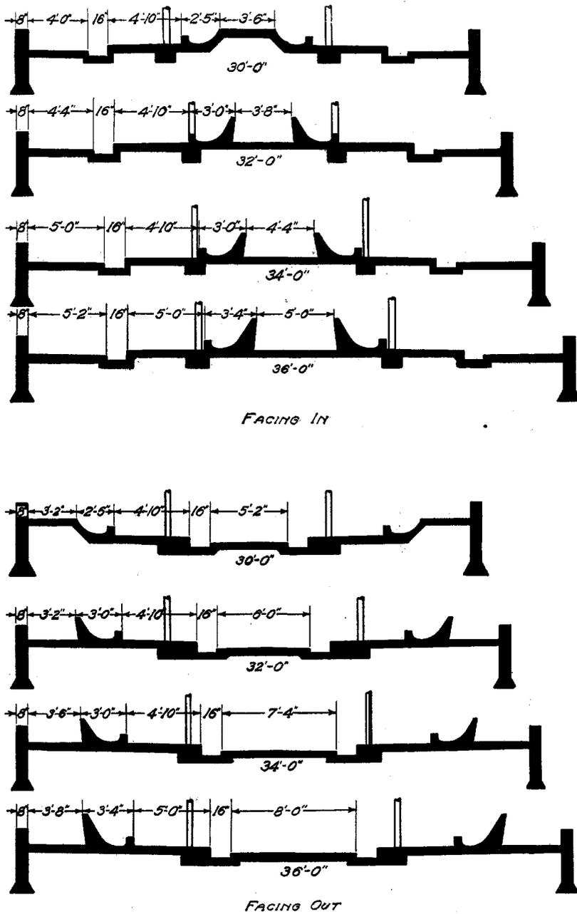
FIG. 6.—Typical sections showing plan for cows facing in or cows facing out in barns of different widths. A 34-foot width is a very common one, though a 32-foot width is often used with satisfaction. (Refer to figure 16 for correct stall length for different breeds.)
