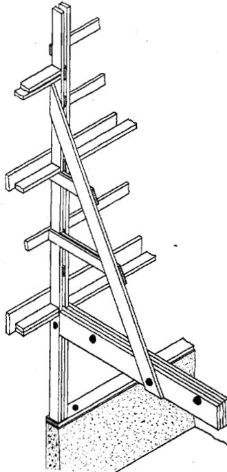
FIG. 14.—Girder and end wall construction.
