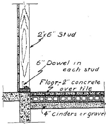
FIG. 28.—A grain bin, showing floor and wall construction. Bin floors should be dry and rat-proof. The walls should be well anchored to resist the thrust of several feet of grain.
