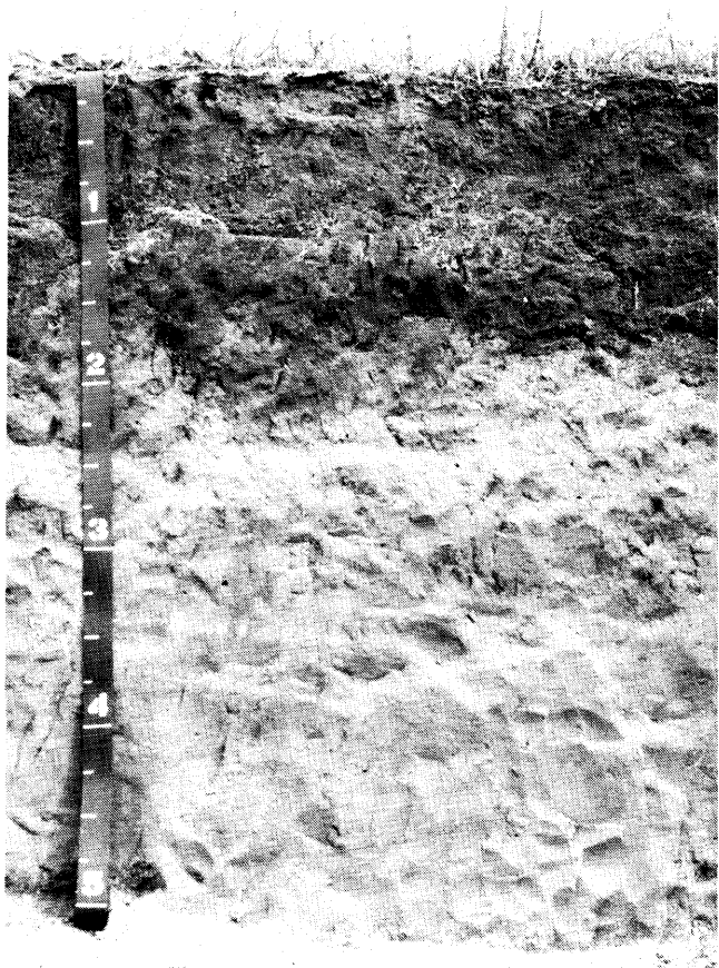
Figure 4. A Naron fine sandy loam located in Rice County: 0-14 inches fine sandy loam, 14-40 sandy clay loam, and 40-60 fine sandy loam. (Soil Conservation Service photo)
