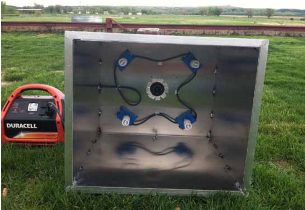
Figure 1. Internal view of the light box showing the wiring and light bulb placement.
