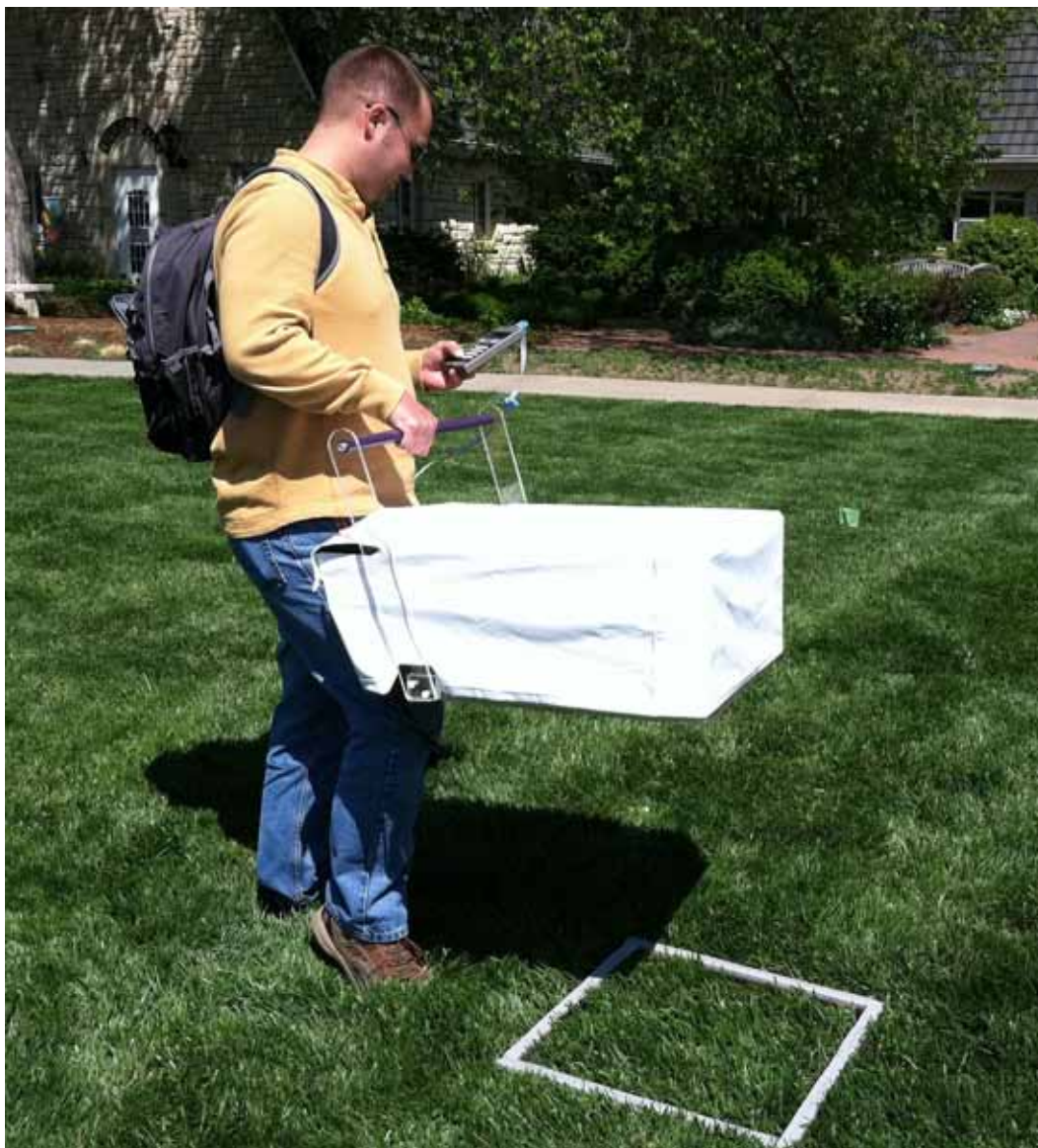
Figure 3. The new fabric cover facilitates dark measurements.
