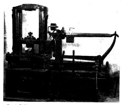
FIG. 4. Richle testing machine used in determining the breaking strength of bones. This particular machine is a part of the equipment in the Division of Engineering of Kansas State College.
