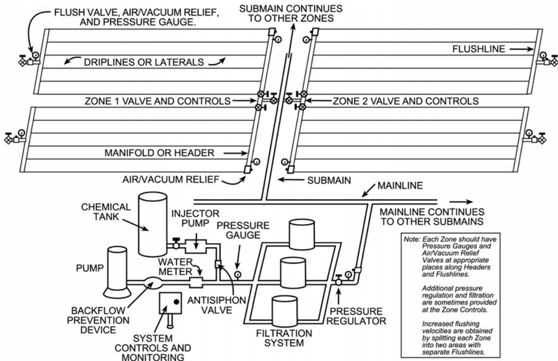
Figure 2. Layout for a well-designed SDI system (Lamm and Camp, 2007).
