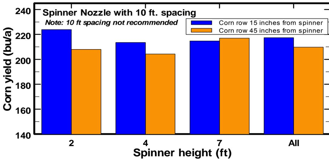
Figure 11. Row-to-row variations in corn yields as affected by sprinkler height for 10 ft. spaced in-canopy sprinklers. Sprinkler lateral travel direction was parallel to crop rows. Data was averaged from four irrigation levels for 1996 to 2001, KSU Northwest Research-Extension Center, Colby, Kansas.
