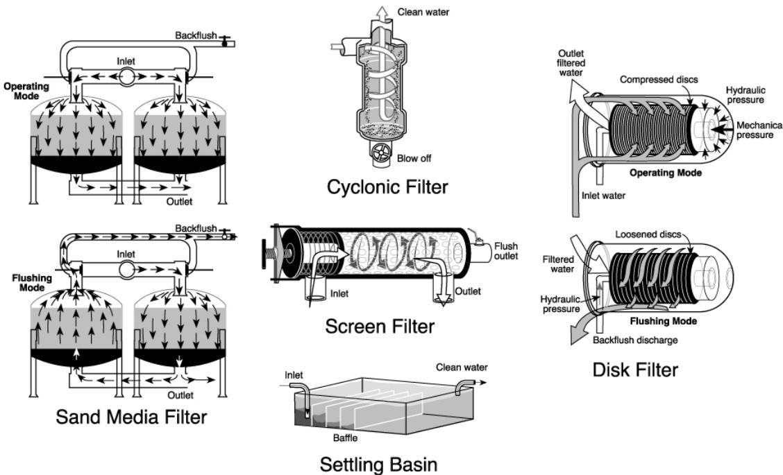
Figure 4. Schematic description of various filtration systems and components.
