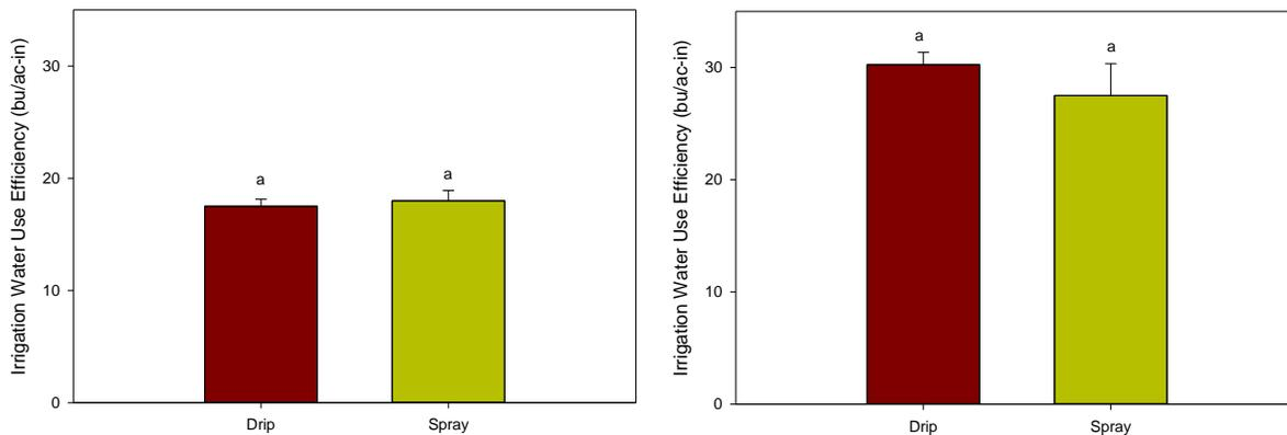
Figure 3. Irrigation water use efficiency of Mobile Drip Irrigation (Drip) and Low Elevation Spray Application (Spray) for irrigation capacity of 2.3 gpm/ac during the 2015 growing season at the Kansas State University Southwest Research-Extension Center, near Garden City, Kansas.
