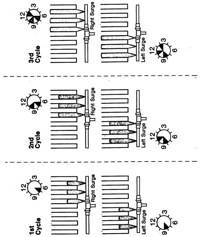
Surge valve in the middle of two sets of gated pipes. FIGURE 1.
