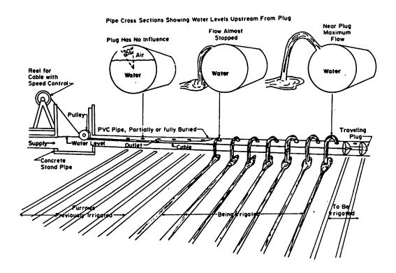
FIGURE 3. Layout and components of a cablegation system (Kemper  $\underline{\text{et}}$   $\underline{\text{al.}}$ , 1983).
