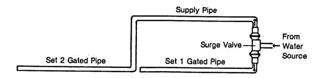
FIGURE 4. Locating the surge valve at the upper end of the field.
