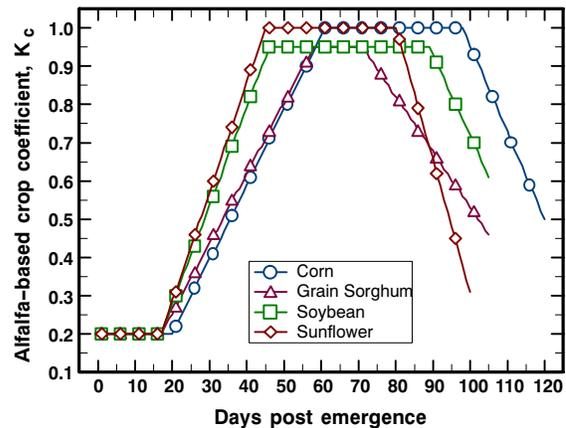
Figure 1. Alfalfa-based crop coefficients used in the simulated irrigation schedules and crop yield modeling.
