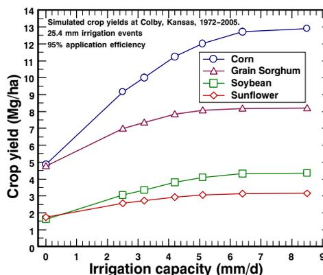
**Figure 3. Simulated summer crop yields in relation to irrigation system capacity for the 34 years, 1972 to 2005, Colby, Kans.**
