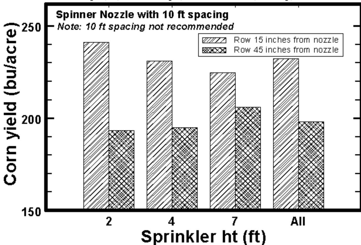
**FIGURE 3.** Row-to-row variation in corn yields as affected by sprinkler height when in-canopy sprinklers are too widely spaced at 10 ft. Note: Field average yield for a particular sprinkler height would be the average of the two side-by-side bars rather than the higher yield that could be obtained with properly spaced in-canopy sprinklers.
