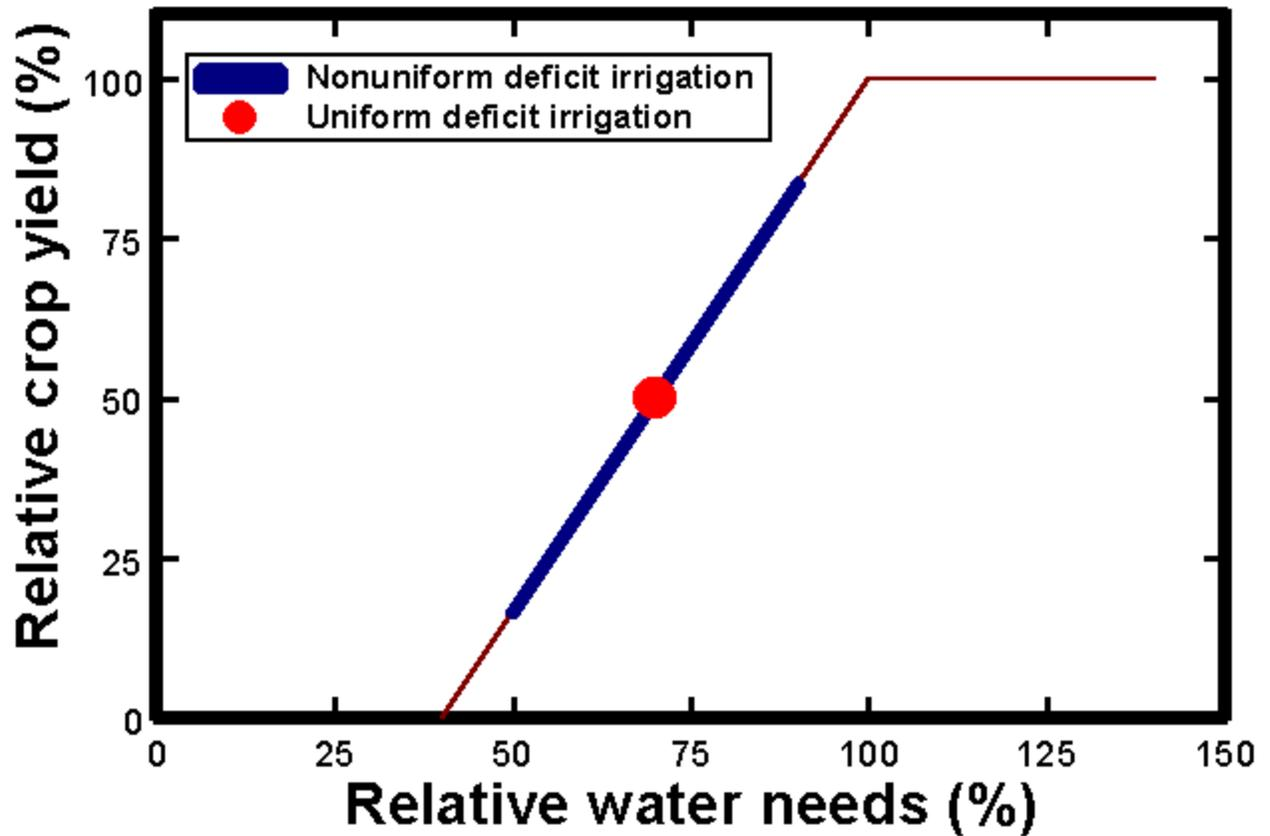
**Figure 2.** Hypothetical relationship of relative crop yield and relative water needs for nonuniform deficit irrigation (bold range bar) and for uniform deficit irrigation (large dot). Average relative water need is the same for both irrigation schemes, and, consequently, the average relative yield would also be the same.
