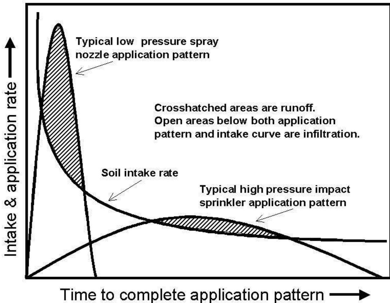
**Figure 1.** Typical soil intake and sprinkler application patterns as related to time to complete the whole application pattern. Note: Increasing or decreasing the center pivot sprinkler travel speed would not change the peak application rate for either sprinkler type. Thus runoff would likely still occur. Increasing or decreasing the travel speed would change the duration of the pattern and thus would decrease or increase the total amount of runoff.
