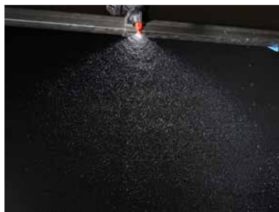
Figures 1-3. These images show the difference in droplet size based on the type of nozzle selected. Nozzle: AIXR 11004 (air inclusion 110-degree flat fan coarse spray); XR11004 (flat fan medium/fine spray); and TT104 (Turbo Teejet Extra coarse spray). Photo: Mark Ledebuhr, Application Insights, LLC 2020, www.bugwood.org
