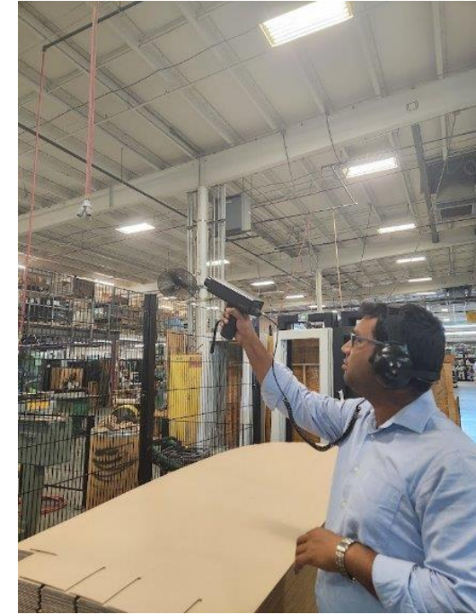
PPI Intern using the ultrasonic leak detector
